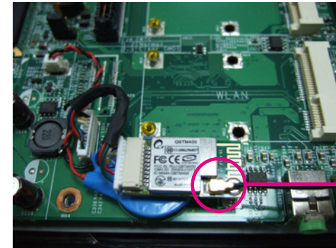
Attach RF cable to the module
