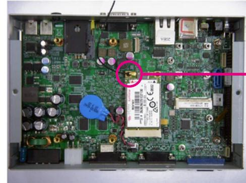
Attach RF cable to the module
