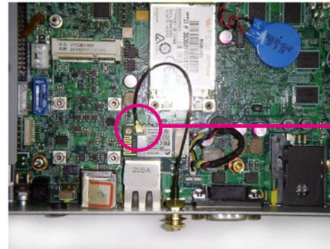
Attach RF cable to the module
