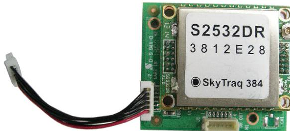
The S2532DR GPS Dead-Reckoning receiver module combines GPS position data, gyroscope data (measuring turning angle), and odometer data (measuring distance traveled) to formulate position solution. This enables accurate navigation solution in poor signal environment or signal blocked area such as inside tunnels. The S2532DR is ideal for applications requiring accurate continuous navigation with 100% availability.
