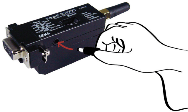
Figure 2-2 Connecting Power to Parani-SD1000
