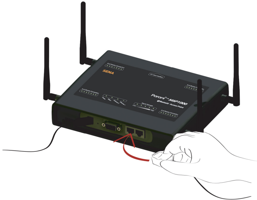
Figure 2-3 Connecting a network cable to the Parani-MSP1000
