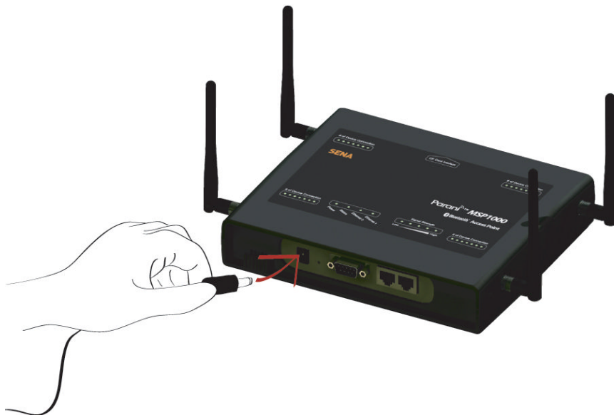
Figure 2-2 Connecting the power to the Parani-MSP1000
