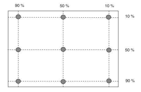
**Note 3:** The luminance uniformity of 9 points is defined by dividing the maximum luminance values by the minimum test point luminance
