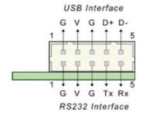
Figure 5.1 Board mounted header
