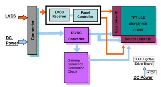
Figure 1.1 Function Block Diagram
