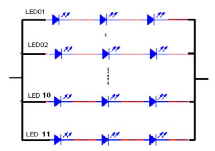
**Note 3:** The LED Light Bar power consumption variance is 10%. Calculator value for reference ( $IL \times VL = PLED$ )
