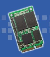
With its compact size, high performance and conformity with JEDEC standard MO-300A, the mSATA Industrial Grade Embedded Module is ideal for mission-critical embedded storage applications that have space constraints and require high performance and reliability. The mSATA design is based on the JEDEC standard MO-300A with the ubiquitous SATA-II, 3 Gbps interface. Measuring only 2.0 x 1.2 inches (50.8 x 29.8 mm) mSATA SSDs are extremely compact and lightweight.
