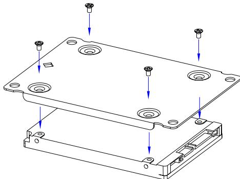
Step 4: Fasten the four screws to install the HDD and HDD Bracket to the chassis, then connect the SATA cable to the HDD.
