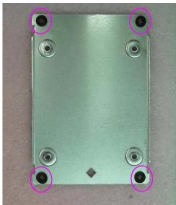
Step 3: Fasten the four screws to fix the HDD and HDD bracket
