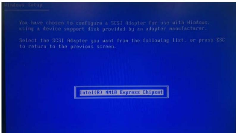
Step 10 – The following messages will appear on the screen. Press “S” to specify additional SCSI adapters. Press “ENTER” and Windows Setup will continue to install OS.
