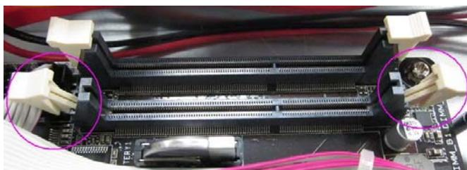
Step 3: Line up the pins and firmly (but not roughly) press on the outside of Memory Card to install.
