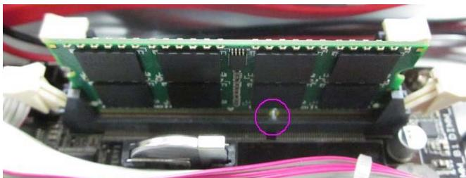
Step 4: Snap the DIMM slot tabs shut, locking the Memory Card in place.
