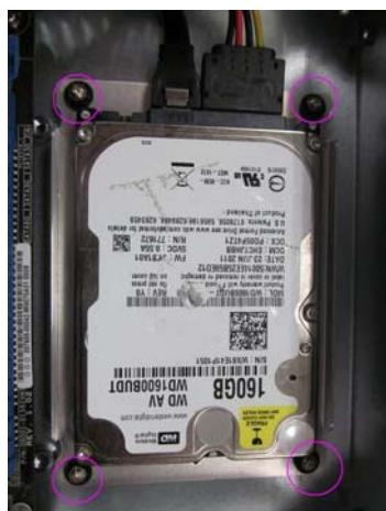
Step 5: Close the cover of the AEC-6643 and fasten the screws and copper cylinders.
