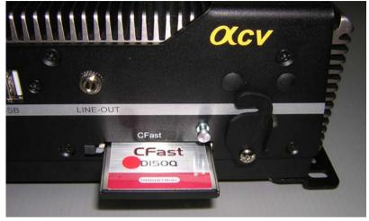
Step 4: Fasten the cover of the CFast<sup>™</sup> card.
