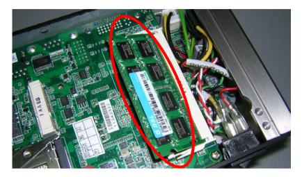
Step 6: Press the SDRAM and make sure that it has been inserted properly.
