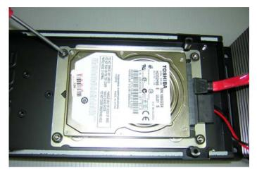
Step 8: Fasten the bottom HDD kit case of AEC-6613.
