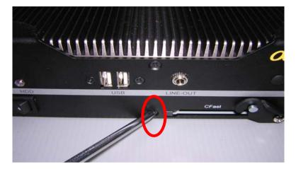
Step 4: Loosen the screws on the rear panel of AEC-6613
