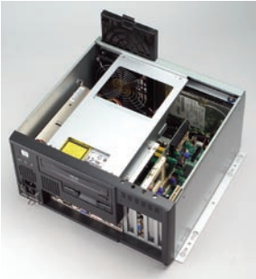
Solid disk drive housing & easy-to-maintain fan filter
