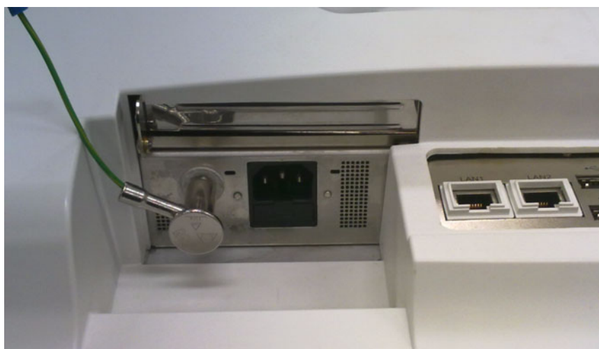
Figure 2.10 POC-227 Equipotential terminal connected with grounding cable
