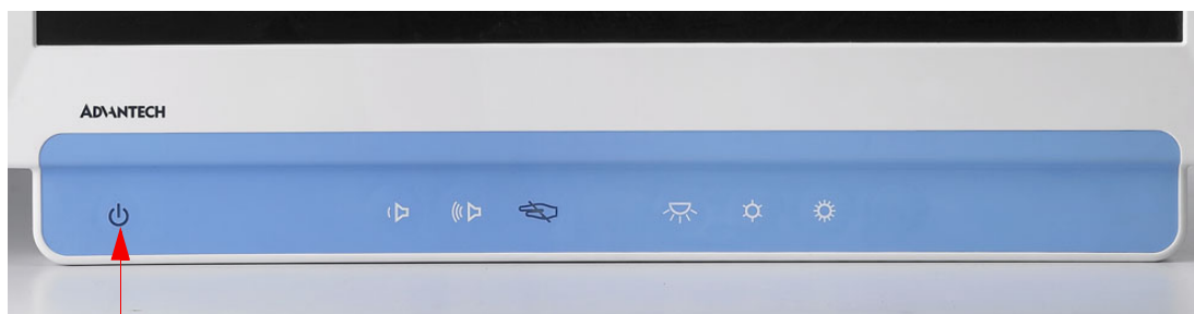
Figure 2.11 Press the power button to boot system
