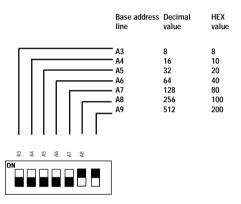
Note: On the PCM-3641 the address line A9 does not appear on the DIP switch as it is permanently hardwired to HEX 200 on the card.
