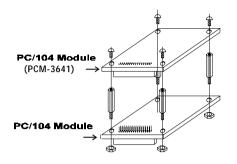
2. Screw the PCM-3641 to the brass spacer. This completes the hardware installation.
