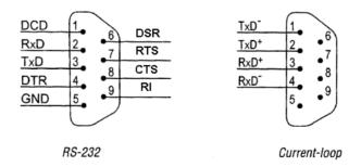
Figure 5.2: PCL-741 Pin Assignments
