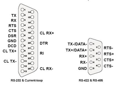
Figure 5.1: PCL-740 Pin Assignments
