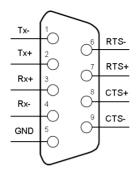
Figure 5.8: PCL-746+ RS-422 DB-9 Pin Assignments
