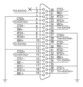
Figure 5.6: PCL-746+ RS-422/RS-485 DB-37 Pin Assignments
