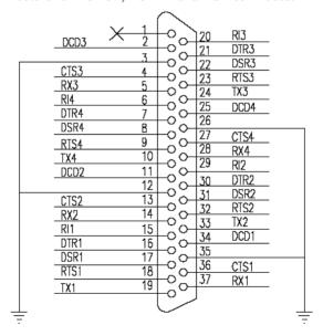
Figure 5.3: PCL-746+, PCL849A/B/+/L RS-232 DB-37 Pin Assignments
