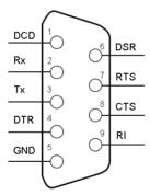
Figure 5.5: PCL-746+, PCL849A/B/+/L RS-232 DB-9 Pin Assignments
