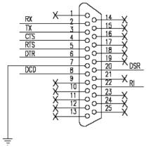
Figure 5.12: PCL-858A/B with OPT8A+RS-232 DB-25 Pin Assignments
