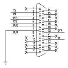
Figure 5.13: PCL-858A/B with OPT8B+/C RS-232 DB-25 Pin Assignments
