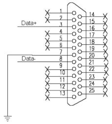
Figure 5.9: PCL-746+ RS-485 DB-25 Pin Assignments
