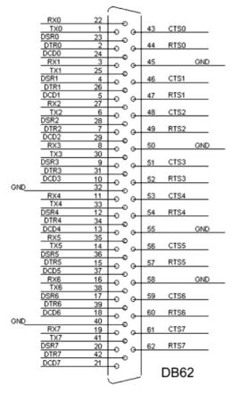
Figure 5.11: PCL-858A/B RS-232 DB-62 Pin Assignments
