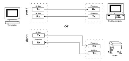
Figure 2.13: Current Loop Link
