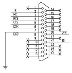
Figure 5.4: PCL-746+, PCL849A/B/+/L RS-232 DB-25 Pin Assignments
