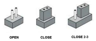
Figure 2.9: Jumper Setting
