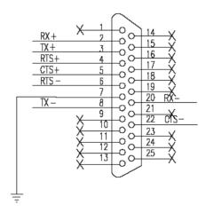
Figure 5.7: PCL-746+ RS-422 DB-25 Pin Assignments
