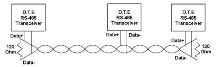
Figure 5.15: RS-485 Wiring Topology
