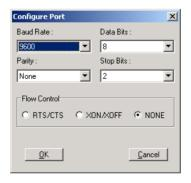
In the **Configure Port** dialog box, you can configure the Baud Rate, Data bits, Parity, Stop Bits and the flow control mode for that specific port (or for all ports). After you have configured all the settings you want to change, click OKto make this configuration active.
