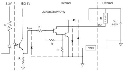
Figure 3.9: Isolated Digital Output Connection
