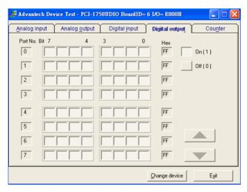
Figure 2.9: The Test Diagram Box for Digital Output
