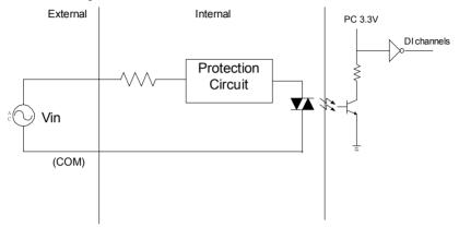
Figure 3.8: Isolated Digital Input Connection
