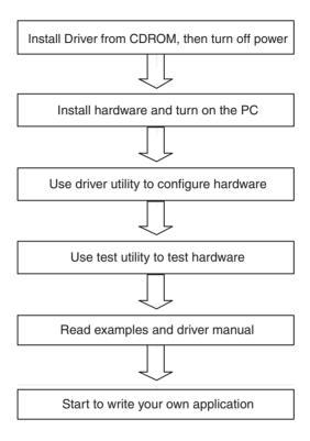
Figure 1.1: Installation Flow Chart
