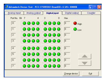
Figure 2.8: The Test Diagram Box for Digital Input
