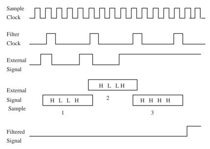
Figure 4.2: Digital Filter Example
