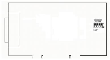
Figure 3.5: Location of DIP Switch on PCI-1758UDI
