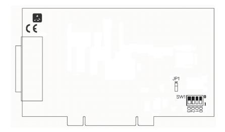
Figure 3.6: Location of DIP Switch and Jumper on PCI-1758UDO
