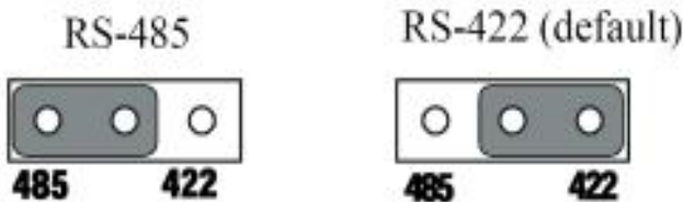
Figure 2.22: RS-422/485 Selection by Jumper Setting
