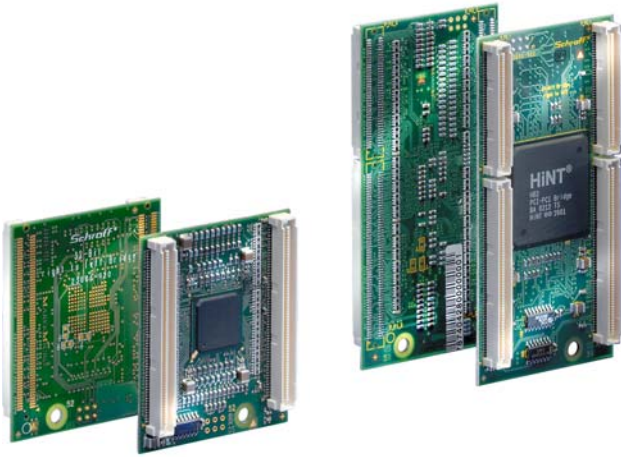
Photo shows 32-bit and 64-bit bridges
