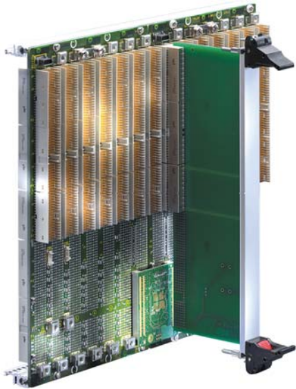
Photo shows primary and secondary backplane with inserted bridge and fitted rear transition board
