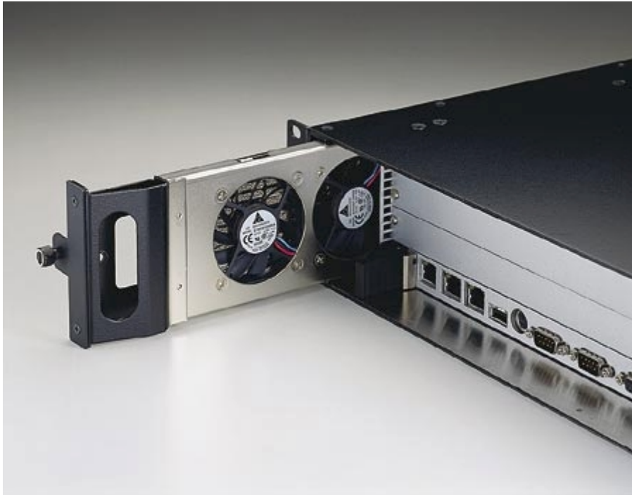
Figure 2-5: Hot swappable fan maintenance
