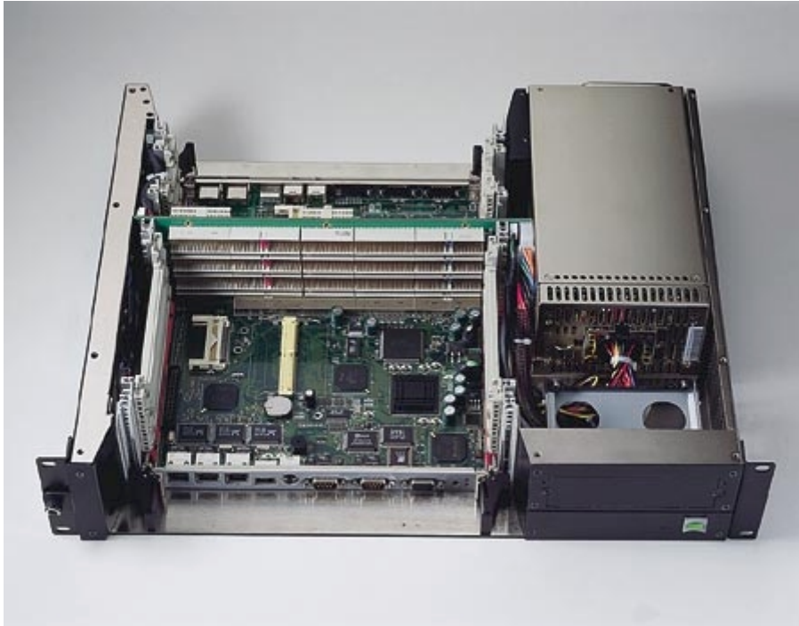
Figure 2-2: Board integration of MIC-3056
