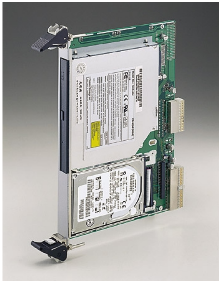
Figure 2-4: Installing 2.5" hard disk drives and slim CDROM
