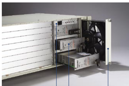
LED board Hot-swappable 193-CFM fan module AC or DC cPCI 500 W + 250 W redundant (2+1) power supplies
