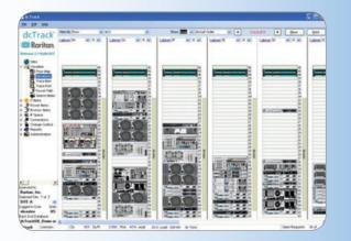
**dcTrack** – Using Raritan's intelligent Asset Management Tags (AMT) and Asset Management Sensors (AMS), EMX provides real-time asset location to dcTrack, Raritan's data center infrastructure management (DCIM) software providing accurate asset location tracking to the 1U level in a rack. Feature ports support Raritan's electronic asset tagging to track assets in 1U rack increments
