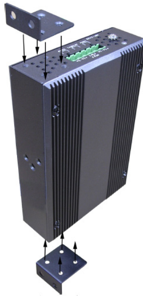
Figure 2.15 Combine the Metal Mounting Kit
