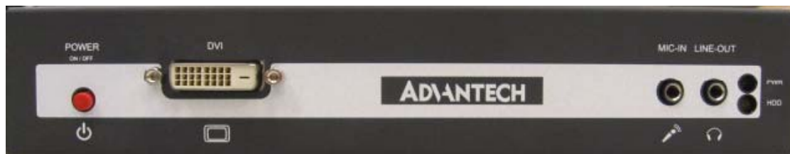
Figure 2.1: DSA-3300 front metal face plate external I/O connectors
