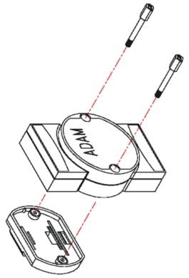
Figure 2.5: DIN Rail Mounting
