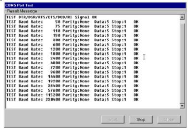
Figure 3.17: Loopback Test
