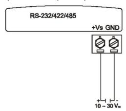
Figure 2.7: Power Connection for ADAM-4570W/4571W
