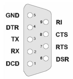
Figure 2-1 RS-232 Terminal (DTE) connections
