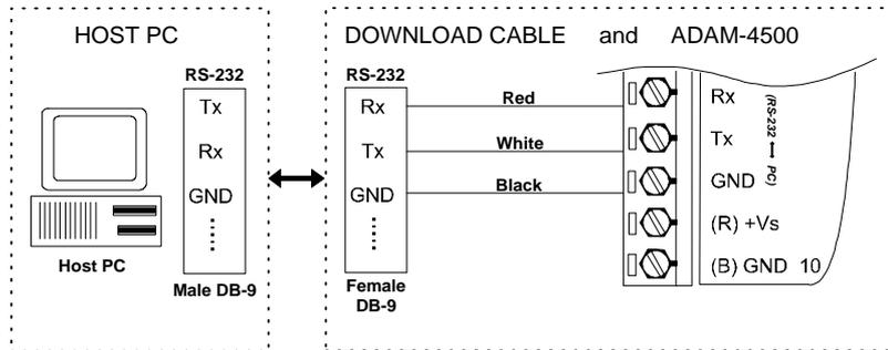
**Figure 2-1: Download Cable Connections**
