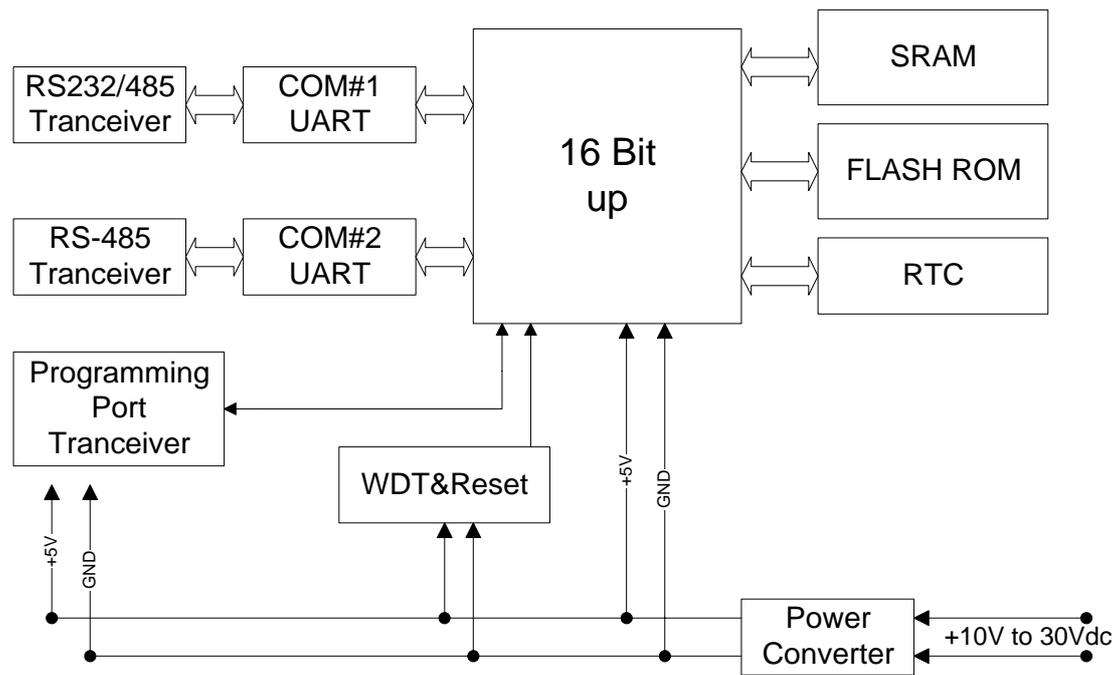
**Figure 1-2: ADAM-4500 Function Block Diagram**
