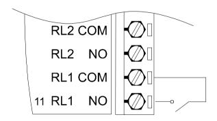
Figure 3-63 ADAM-4060 Form A Relay Output Wiring Diagram
