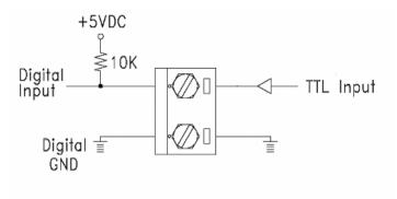
Figure 3-41 ADAM-4050 TTL Input Wiring Diagram
