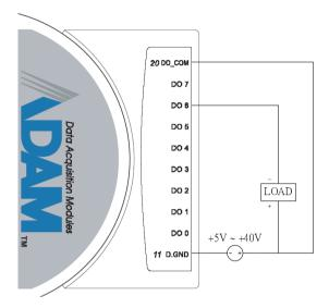
Figure 3-58 ADAM-4056S Digital Output Wiring Diagram
