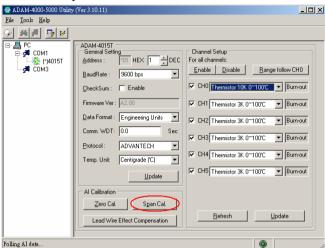
Apply 30K ohms resistor with 0.01% accuracy to CH0 and then Click on "Save"
