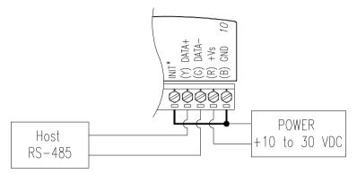
Figure 2-3 Grounding the INIT\* Terminal
