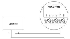
Figure 8-7 Setup for Voltage Output Calibration
