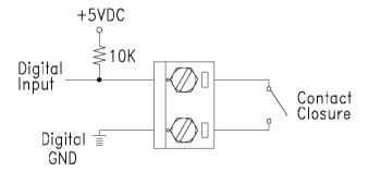
Figure 3-8 ADAM-4011/4011D Digital Input Wiring Diagram
