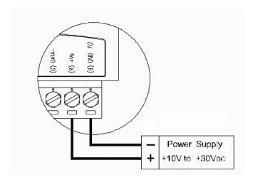
Figure 2-1 Power Supply Connections
