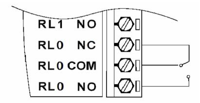
Figure 3-68 ADAM-4069 Form C Relay Output
