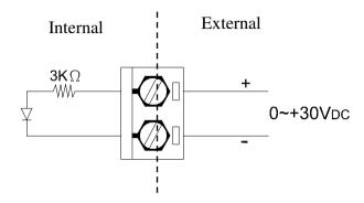
Figure 3-48 ADAM-4052 Isolation Digital Input Wiring Ground
