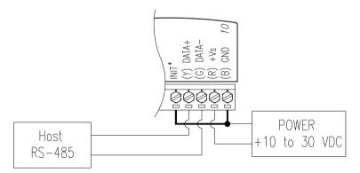
**4. Move hardware switch to Initial mode** (For some older Adam models, use an external wire to connect the INIT\* terminal to the GND terminal. Booting the module while connecting the INIT\* terminal with the module's GND terminal forces the configuration into a known state called the INIT\* state.)
