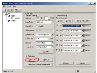
Apply 800.0 ohms resistor with 0.01% accuracy to CH0 and then Click on "Save"
