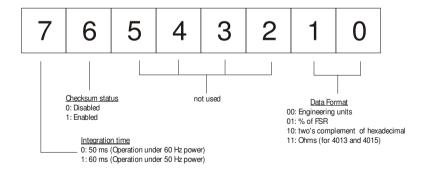
Figure 5-1 *Data format for FF (8-bit parameter)*
