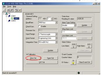
Figure 8-2 Zero Calibration
