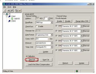
Apply 200.0 ohms resistor with 0.01% accuracy to CH0 and then Click on "Save"
