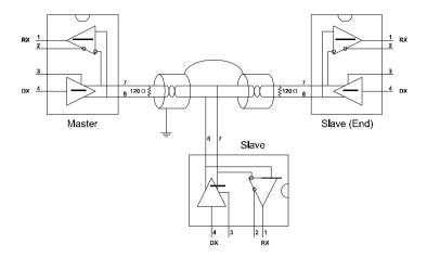
Figure E-5 Termination resistor locations
