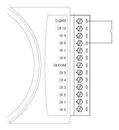
Figure 3-45 ADAM-4051 Dry Contact Wiring Diagram
