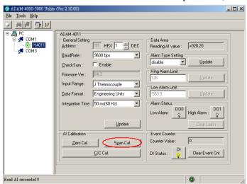
Figure 8-3 Span Calibration
