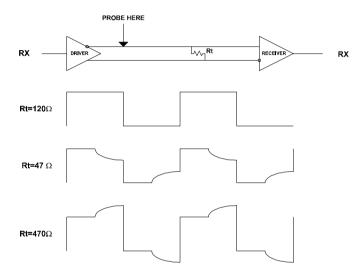
Figure E-4 Signal Distortion
