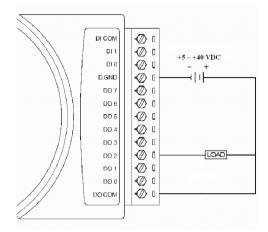
Figure 3-53 ADAM-4055 Digital Output Wiring Diagram
