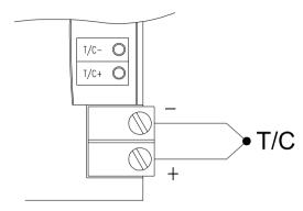
Figure 3-3 ADAM-4011/4011D Thermocouple Input Wiring Diagram
