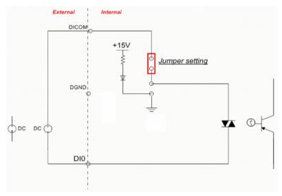
Figure 3-55b ADAM-4055 Digital Input Wet Contact Diagram (Internal)
