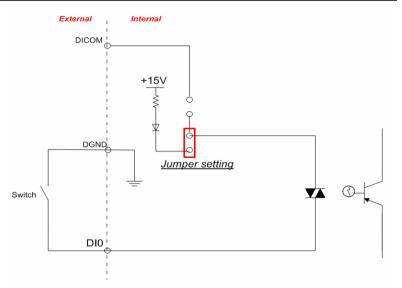
Figure 3-54b ADAM-4055 Digital Input Dry Contact Diagram (Internal)
