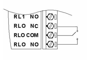
Figure 3-65 ADAM-4068 Form C Relay Output Wiring Diagram
