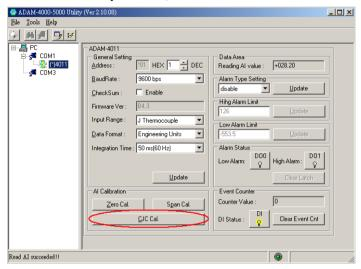
Figure 8-4 Cold Junction Calibration
