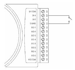
Figure 3-54a ADAM-4055 Digital Input Dry Contact Wiring Diagram
