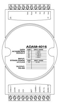
Figure 3-21 ADAM-4016 Analog Input/Output Module
