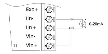
Figure 3-23 ADAM-4016 Strain Gauge Current Input Wiring Diagram
