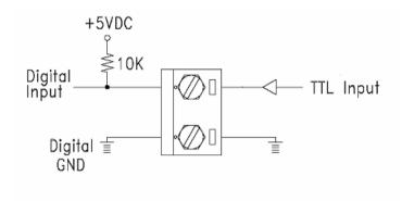
Figure 3-13 ADAM-4012 Digital Input Wiring Diagram Used with TTL
