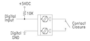
Figure 3-14 ADAM-4012 Digital Input Wiring Diagram
