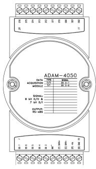
Figure 3-40 ADAM-4050 Digital I/O Module
