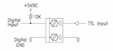
Figure 3-7 ADAM-4011/4011D Digital Input Wiring Diagram
