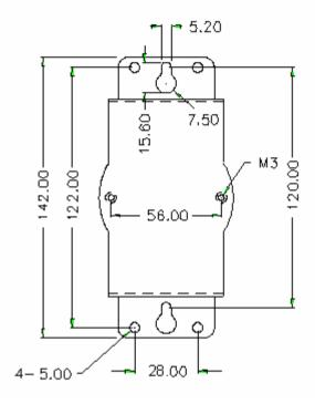
Figure C-4 Panel Mounting Bracket Dimensions
