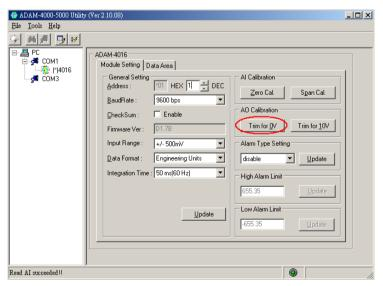
Figure 8-8 Zero Calibration
