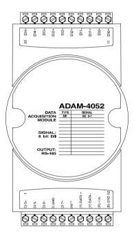
Figure 3-47 ADAM-4052 Isolated Digital Input Module
