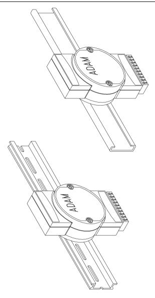
Figure C-3 DIN-Rail Mounting
