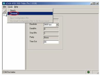
Figure D-3 Terminal Function
