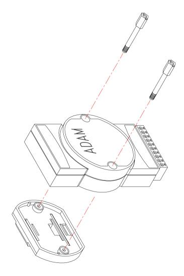
Figure C-2 DIN-Rail Adapter
