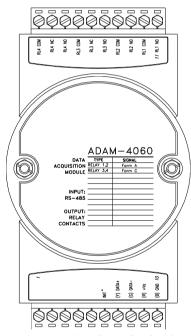
Figure 3-61 ADAM-4060 4-channel Relay Output Module
