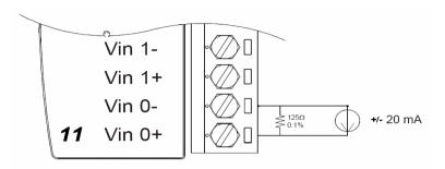
Figure 3-30 Current Input Wiring Diagram of ADAM-4017
