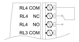
Figure 3-64 ADAM-4060 Form C Relay Output Wiring Diagram
