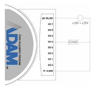
Figure 3-60 ADAM-4056SO Digital Output Wiring Diagram
