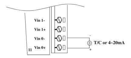
Figure 3-33 ADAM-4018+ Thermocouple Input Wiring Diagram
