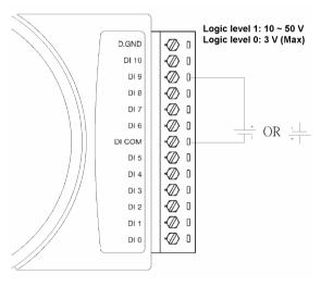
Figure 3-46 ADAM-4051 Wet Contact Wiring Diagram
