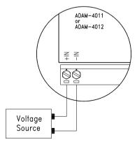
Figure 8-1 Applying Calibration Voltage
