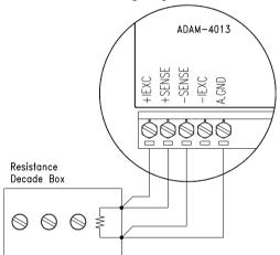
Figure 8-5 Applying calibration resistance
