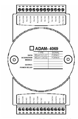
Figure 3-67 ADAM-4069 Relay Output Module
