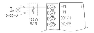
Figure 3-5 ADAM-4011/4011D Process Current Input Wiring Diagram
