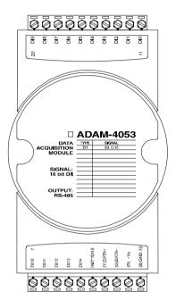
Figure 3-49 ADAM-4053 16-channel Digital Input Module
