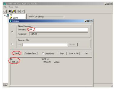
Figure D-4 Terminal Function
