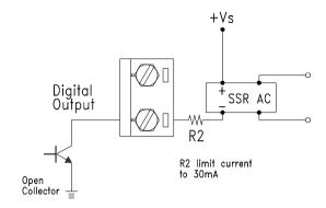
Figure 3-6 ADAM-4011/4011D Digital Output Wiring Diagram
