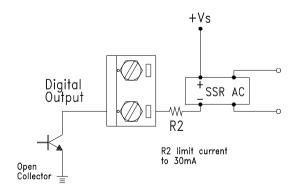
Figure 3-12 ADAM-4012 Digital Output Wiring Diagram
