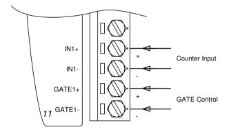
Figure 3-73 ADAM-4080/4080D Photo-isolated Input
