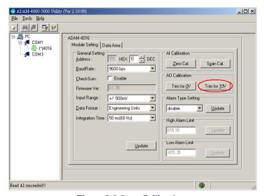
Figure 8-9 Span Calibration
