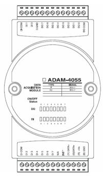
Figure 3-52 ADAM-4055 16-channel Digital I/O Module
