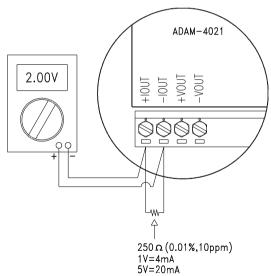
Figure 8-6 Setup for Analog Output Calibration
