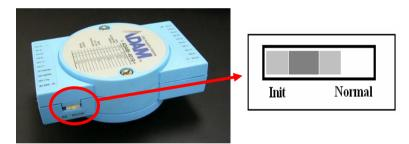
Figure 2-4 Set INIT switch to "Init"
