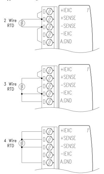
Figure 3-16 ADAM-4013 RTD Inputs Wiring Diagram
