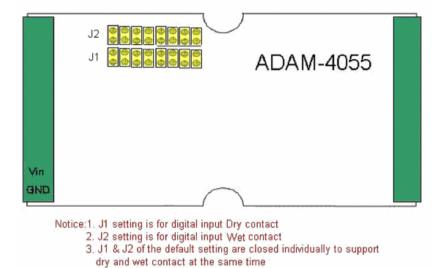
Figure 3-56b ADAM-4055 Default Jumper Setting for the Digital Input Wiring
